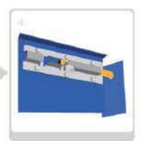
用手搖器把平台調整到適合的工作高度,並用保險銷插入上好安全螺絲帽 Rotate to adjust the platform to a suitable height and locked with the pin to secure in position
