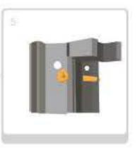
用手搖器把平台調整到適合的工作高度,並用保險銷插入上好安全螺絲帽 Rotate to adjust the platform to a suitable height and locked with the pin to secure in position
