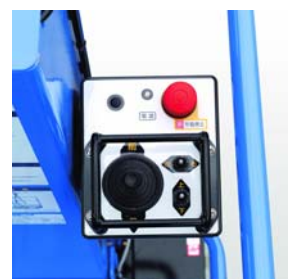
Photo: Upper control box
